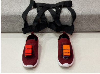
Fig. 1. Wearable sensing system prototype, with the harness and IMU on the belt and a sensing unit (ESP32, IMU, and pressure insole) on each shoe.
